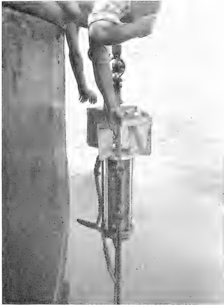
Fig. 1. Probe for measuring temperature gradient. (By courtesy of British Petroleum Co.)
